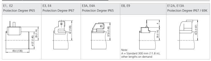
The specified IP rating applies only in the case of correctly connected connectors (male + female) with the corresponding IP rating.
