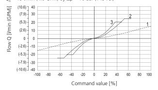
$\Delta \bm{p} = \text{Valve pressure differential (inlet pressure } p_V \text{ minus load pressure } \\ \text{and return pressure } p_T)$
