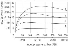
Nominal flow 30 l/min (7.9 GPM)
