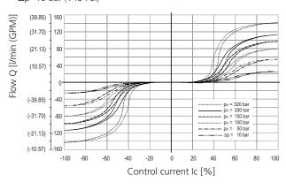
The coil current which initializes the flow through the proportional directional valve can differ due to the production tolerances about in a range of  $\pm$  6% of the limit current.
