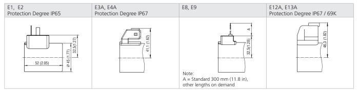
The specified IP rating applies only in the case of correctly connected connectors (male + female) with the corresponding IP rating.
