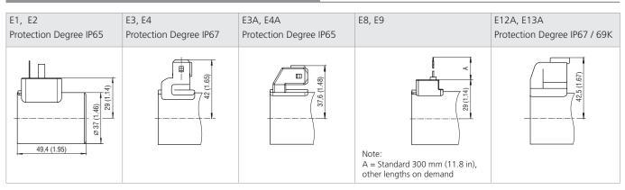
The specified IP rating applies only in the case of correctly connected connectors (male + female) with the corresponding IP rating.
