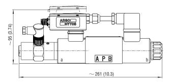
Mounting screws 28.9+1 Nm (6.56+0.7 lbf.ft) M5 x 45 DIN 912-10,9
