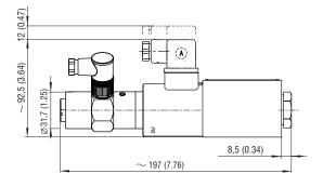
PRMF2-062..../...-...EL7...S0... Valve with one solenoid "a", integrated electronic control unit EL-I\*-1 and position sensor
