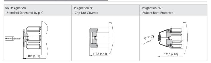
In case of solenoid malfunction or power failure, the spool of the valve can be shifted by manual override as long as the pressure in port T does not exceed 25 bar (363 PSI). For alternative manual overrides contact our technical support.
