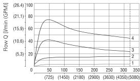
Input pressure p<sub>o</sub> [bar (PSI)]
