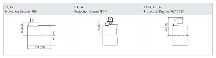
The specified IP rating applies only in the case of correctly connected connectors (male + female) with the corresponding IP rating.
