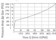
The curve refers to the pressure drop (body part only) with back pressure valve energized to which the pressure drop of the reference spool must be added.
