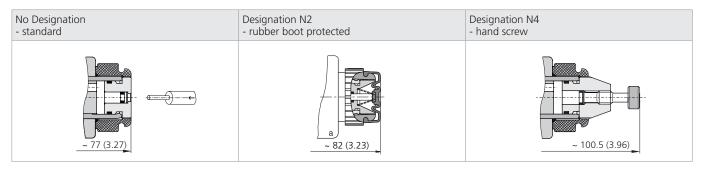
In case of solenoid malfunction or power failure, the valve spool can be shifted by manual override under the condition that the pressure in the back line does not exceed 25 bar (363 PSI). For alternative manual overrides contact our technical support.
