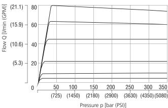
If the pressure resistance increases due to a flow rate increase, the pressure differential also has to increase in order to ensure correct regulation.
