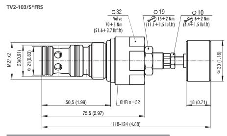
The Blocking function of Pressure compensator is intended for circuits to which can be connected either fix displacement pump or pump with load sensing regulation.
