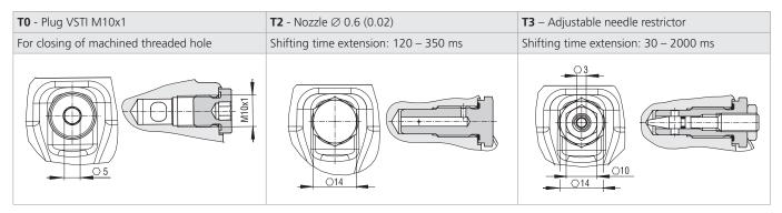
The shifting time is valid at fluid kinematic viscosity  $v = 32 \text{ mms}^{-2}$  and nominal voltage supply. The shifting time depends on translated hydraulic power (product of pressure and volumetric flow).
